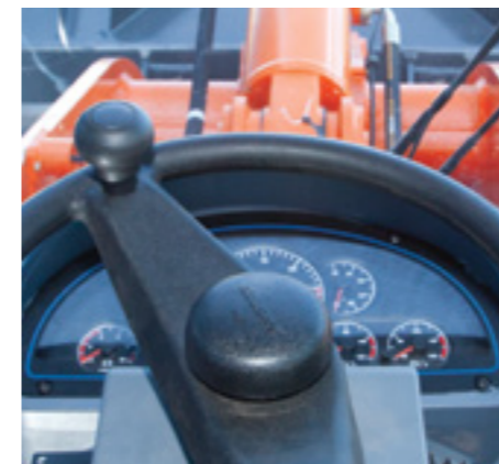
The interior decoration in the cab is upscale : FRP-ABS materials are used for dash board and console and striae treatment is applied to the surface, which is high-grade and durable.
