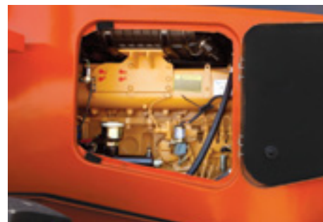
Maintenance windows have been added to each side of the engine hood, thus making daily oil inspection and maintenance works quicker and more convenient.
