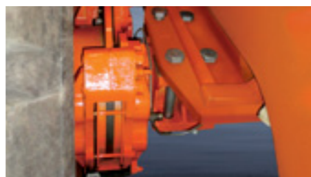
Quickly Changeable Brake Disc Brake disc can be replaced quickly and easily without disassembling tires, deeply shortening the maintenance time and saving time and labor cost.
