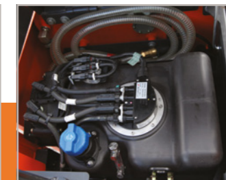
Diesel Exhaust Fluid (DEF) tank
