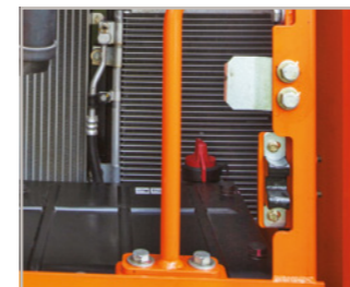
Battery cut-off switch
