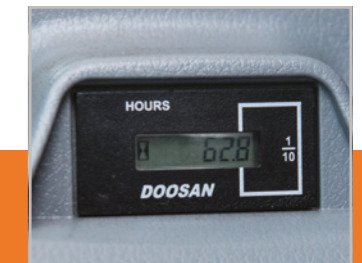
Hour meter (from ground level)
