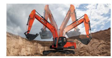
The enhancements to the hydraulic systems of DX220LCA-2 enable you to use engine power in a more effective manner. DX220LCA-2 is capable of performing the same intensity of operations at much lower fuel consumption than others of the same class, significantly increasing your work efficiency.
