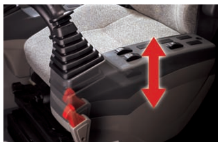
Control stand (Telescopic Function)
