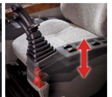
Control stand (Telescopic Function)
