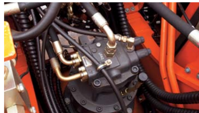
Swing drive Shocks during rotation are minimized, while increased torque is available to ensure rapid cycles.
